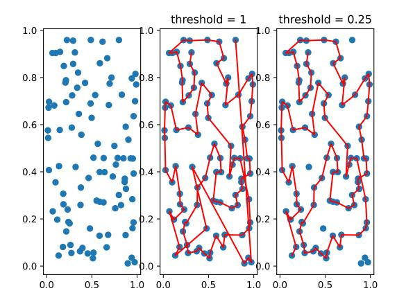
**Parameters closeness\_threshold** (*float*) – The percentile of distances beneath which to consider connecting points, from 0 to 1. Eg. 0.5 would allow points that are closer than 50% of all distances between all points to be connected. Default is 1, which allows all points to be connected.
