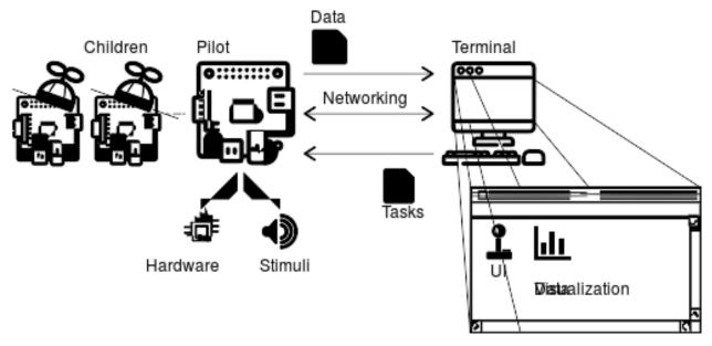
Autopilot performs experiments by distributing them over a network of desktop computers and Raspberry Pis. Each Computer or Pi runs an Autopilot **agent**, like the user-facing *Terminal* or a Raspberry Pi *Pilot*.
