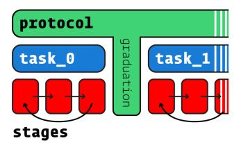
Behavioral experiments in Autopilot consist of *Task* s. Tasks define the parameters, coordinate the hardware, and perform the logic of an experiment.
