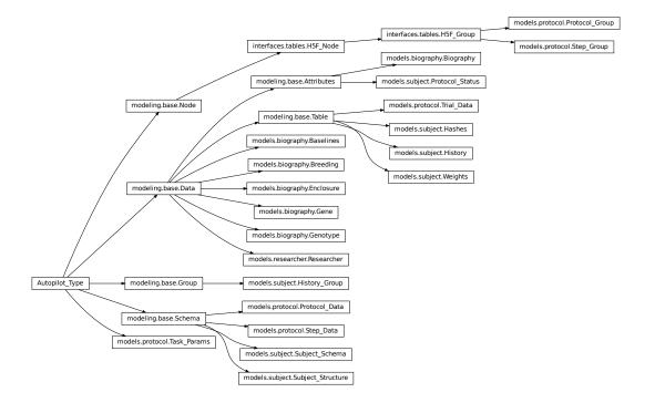
Specific models are then built out of the basic modeling components! This will serve as the point where data models can be added or modified by plugins (stay tuned).
